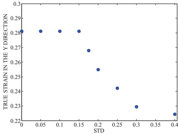
FIG. 3. Plastic strain value corresponding to the local minima in Shannon’s entropy (onset of localization) vs. STD of the different initial distributions of energy. Mean values are calculated for five runs of STD values.
