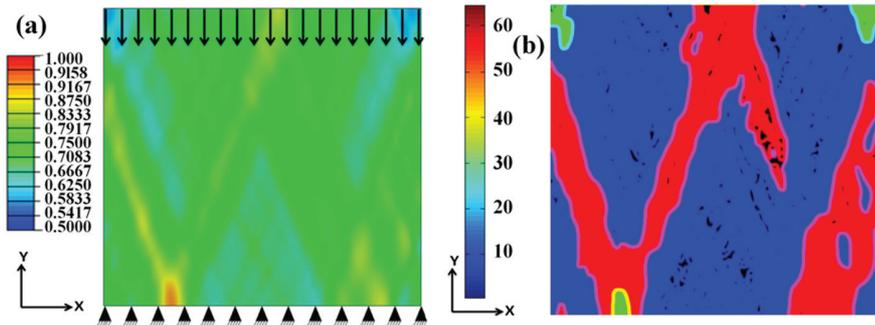
FIG. 1. Model of the plate undergoing dynamic compression. (a) Boundary conditions of prescribed velocity as well as the plastic strain map, projected onto the un-deformed configuration. (b) The corresponding local Shannon's entropies defined on a  $9 \times 9$  pixel local grid. Note the delineation of the localization bands resulting from application of Shannon's entropy.
