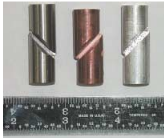
Fig. 2—Photographs of deformed specimens. From left to right: annealed Ti-6Al-4V titanium alloy, commercial OFHC copper and 6061-T351 aluminum alloy. The shear dominated deformation of the gage section is noticeable.
