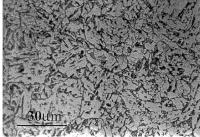
Figure 1. Typical tempered bainitic microstructure of the investigated steel. Etchant: Nital 3%.
