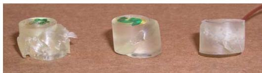
Fig. 8. Failed specimens with shear planes are visible at 45°.
