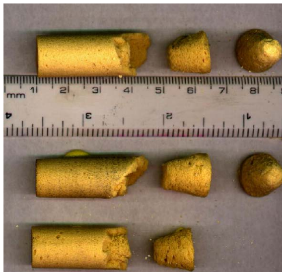
Fig. 2. Broken polyurethane foam projectiles. Note the uniformity of the failure mode: in all the cases, a truncated conical plug is formed.
